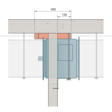
If not possible to fix the lug to the vertical supporting construction above the damper due to space constraints, support the damper by unistrut from min. M8 drop rods, washers and nuts from the horizontal supporting construction. Let the damper rest upon the unistrut, do not fixate. Dimension suspension system acc. to weight and required fire resistance.
